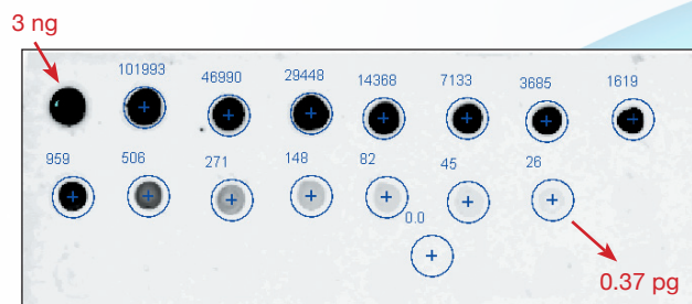
Two-fold serial dilutions of labeled antibody (6 ng to 0.19 pg) were spotted on nitrocellulose and imaged in the 700 nm channel.
